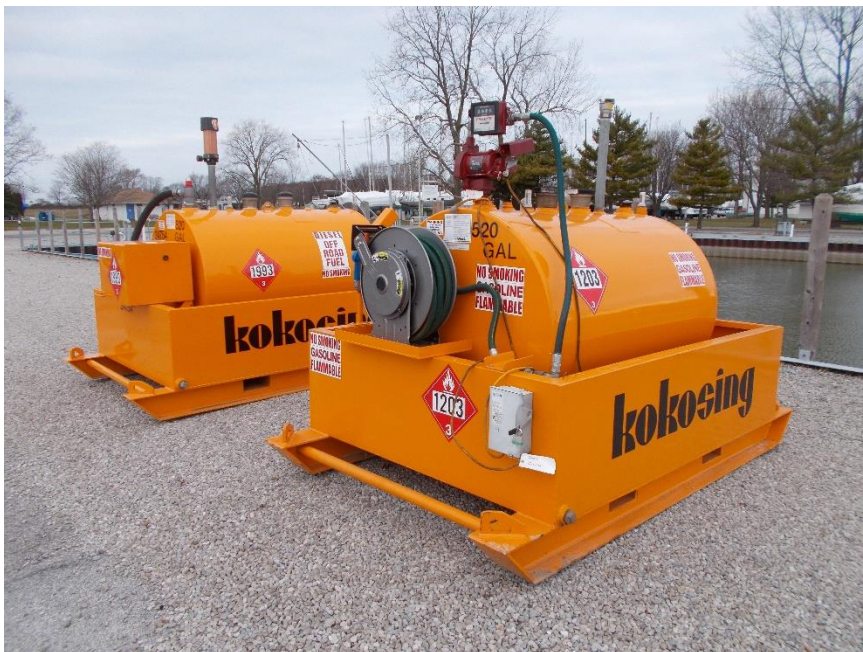
Figure 2: Photo of gasoline and diesel fuel tanks with hose reels and pumps in containment.
