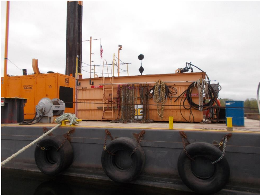
Figure 3: Barge mounted diesel fuel tank in containment.
