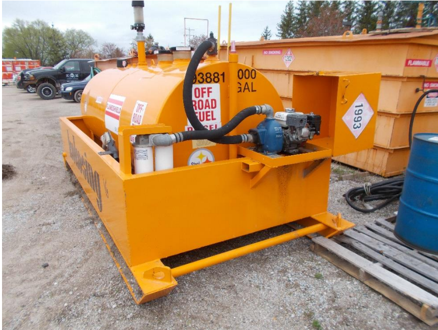
Figure 1: Photo of diesel fuel tank, filters, and pump with delivery hose in containment.
